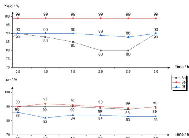
**Scheme 6.** Stereoselective allylation in continuous flow (S6 in the Supporting information for detailed procedure). 3 h buffer time was adopted to ensure a steady-state before data collection.
