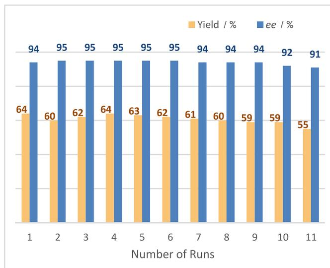
**Scheme 5.** Recycling of heterogeneous catalyst **1h**. For each run, the catalyst was filtered using a medium porosity fritted filter funnel, where 90 mL of DIPEA: THF (1:8) solvent was used for every 1 g of catalyst.
